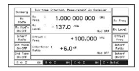
Application mode for intermodulation test on a receiver
