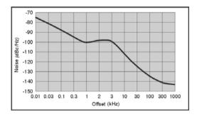
Typical SSB Phase Noise at 1 GHz
