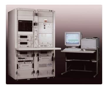
Is the convenience of measuring frequency and power with a single input more important to you than power measurement accuracy? Then the 53150 series of CW Microwave Counters may be for you.
