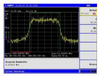
The occupied bandwidth measured in dBc.
