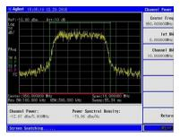
It is quick and easy to set center frequency, integration bandwidth, and channel bandwidth.
