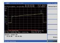
The field strength measurement automatically takes into the account of the antenna factor. The antenna table is definable by the standard N9340B PC software.
