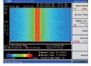
The spectrogram gives the three-dimensional display of power, frequency and time.
