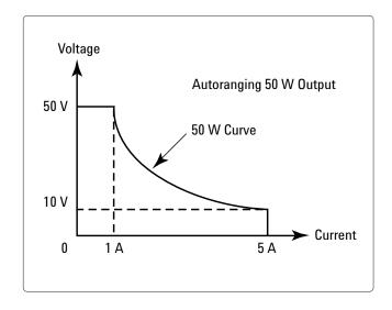
due to its extended voltage and current range, can produce voltage and current combinations in the range of a 250 W non-autoranging power supply.
