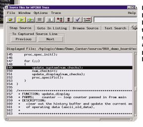
Figure 10. Correlate your logic analyzer trace to the high-level source code that produced it. Easily set up your next logic analyzer trigger by simply pointing and clicking on a line of source code.
