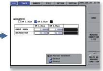
Multi Wavelength Continuous Measurement is a function that allows you to switch the wavelength being measured while keeping the same measurement conditions. This is convenient when you need to measure two wavelengths in a single fiber.
