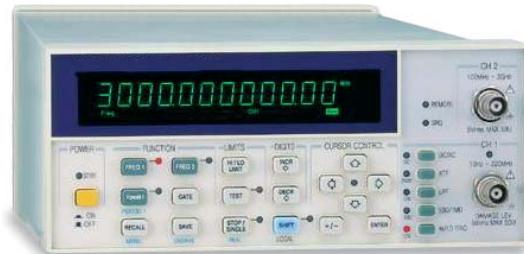
The model **FD-853** is a RF Frequency Counter designed for system and bench use with max 9 digits resolution, featuring RS-232C and GPIB interfaces with full remote control capability. The frequency range is from 10 Hz to 3 GHz and High resolution measurement are possible.
