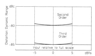
Typical harmonic and intermodulation distortion
