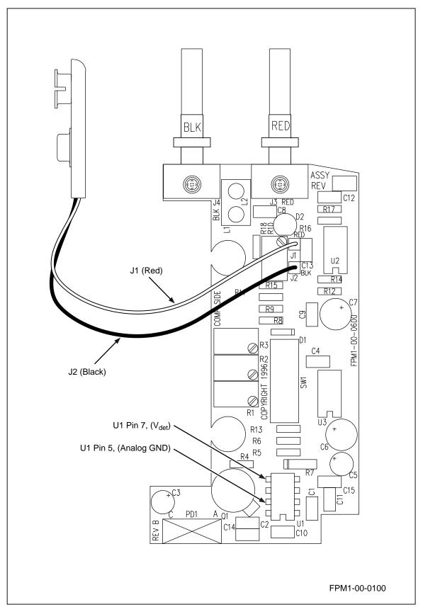
Figure 1. FOM Calibration Measurement and Adjustment Points
