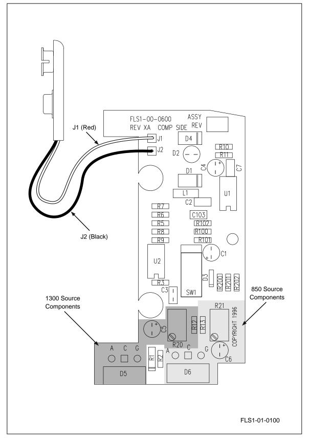
Figure 2. FOS Calibration Adjustment Points
