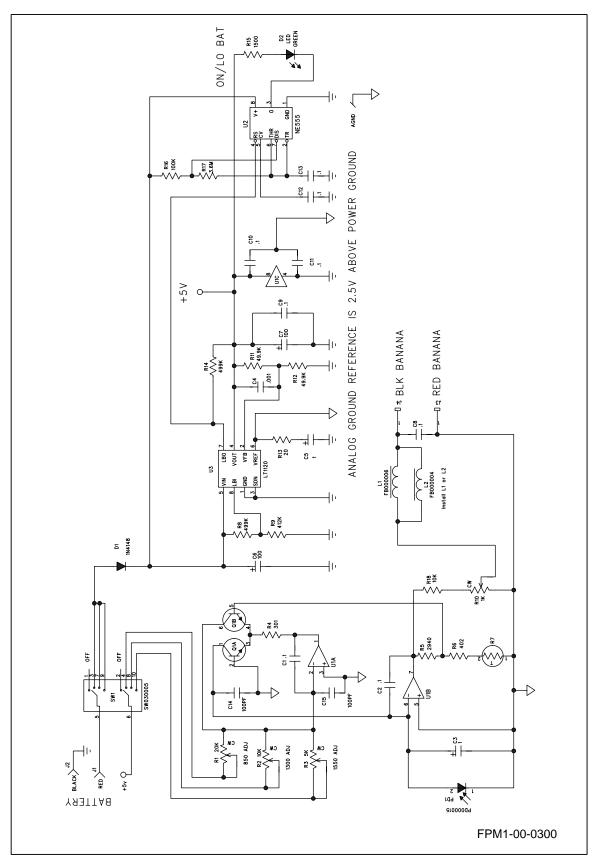
Figure 3. Fiber Optic Meter Schematic
