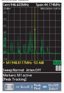
The markers are moved using the navigator buttons and can be set to automatically track to peaks.
