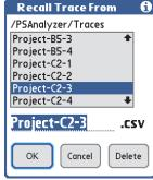
Storage of set-ups allows all of the settings of the instrument to be saved for instant recall to the same instrument, or to another PSA1301T.
