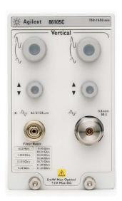
10 Gb SONET transmission has various specified rates depending on the technology being implemented and the network being designed. The OC-192 rate is 9.953 Gb/s. The rate goes up to 10.664 Gb/s with the addition of Forward Error Correction (FEC). In addition there is now OTN G.709, which adds additional network control and further increases the rate to 10.71 Gb/s. To meet this increased transmission speed, components must scale and be tested accordingly.
