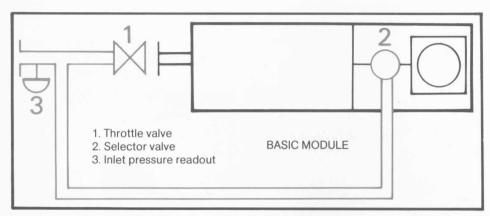
In addition to the basic design concept, ALCATEL ASM 10 and ASM 110 T feature a throttle valve (1), a selector valve (2) and an inlet pressure readout (3) allowing roughing of items of 10 liters (.35 ft<sup>3</sup>) volume.
