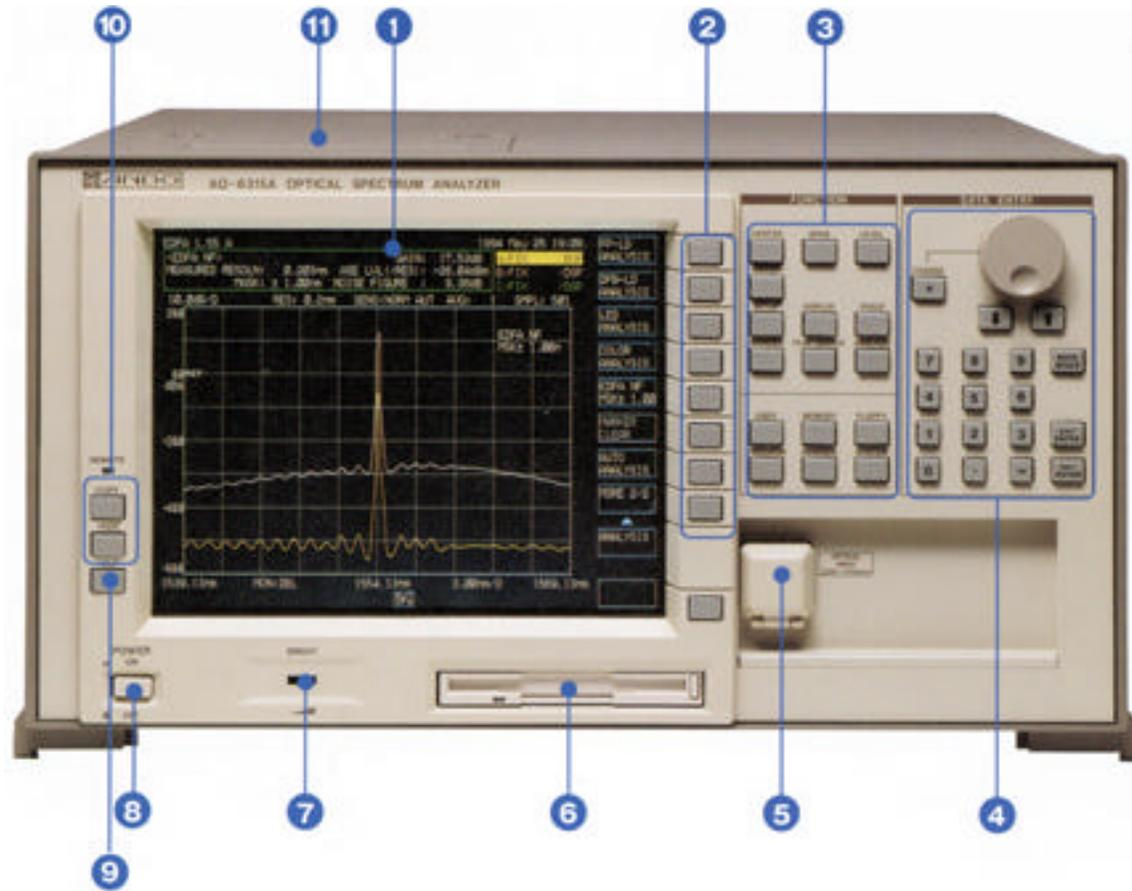
**1-9.4-inch color liquid crystal display** Displays all information such as measurement waveforms, measurement conditions and measured data.
