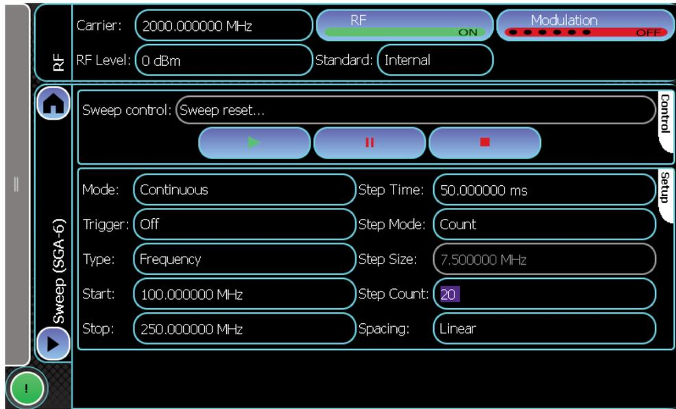
*Typical frequency sweep set-up*
