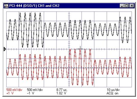
Using baseband sampling, the PCI-444 can measure I/Q communication signals from a 70 MHz I/F strip.
