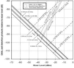
Figure 2. Specified dynamic range for E4407B spectrum analyzer
