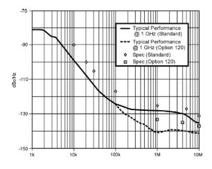
Figure 1. Typical ESA-E Series performance at 1 GHz
