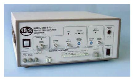
The Trek Model 609E-6-FG High-Voltage Function Generator is a combination of a high-voltage DC-stable power amplifier and a function generator. The high power amplifier is designed to provide precise control of bi-polar output voltages in the range of 0 to ±4 kV DC or peak AC with an output current capability of ±20 mA DC or peak AC. The function generator is capable of generating square, triangle, and sine waveforms in the frequency range of 0.2 Hz to 10 kHz.
