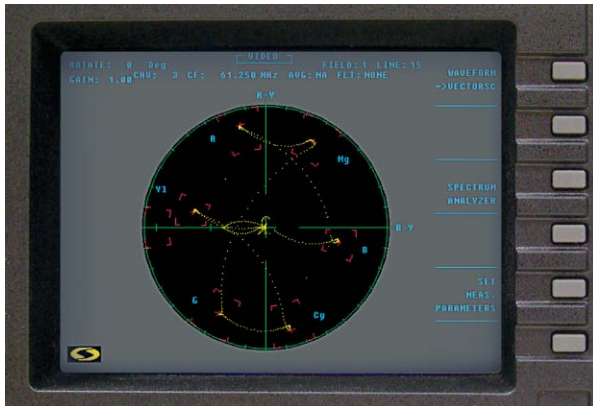
Vectorscope Display of color bars
