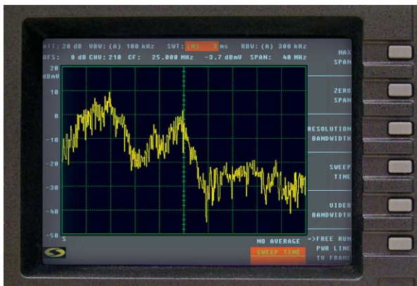
Reverse path ingress is easily captured with high speed scan
